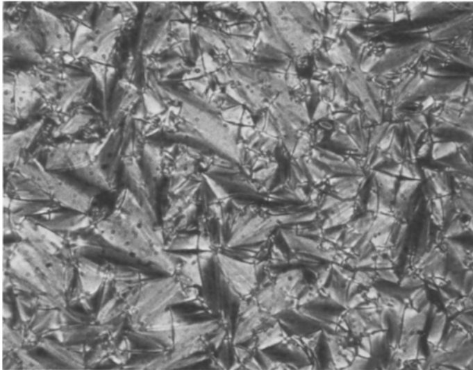
Figure 3: Typical optical polarization micrographs (magnification, 300 x ) of Poly(V): smectic focal-conic texture obtained after 5 hrs of annealing at 118°C.
